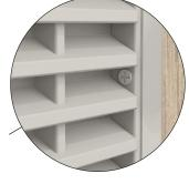
Note: Screw holes based on 400mm square grille. Location and number may vary depending on the size of the grille. Max centres 200mm.
