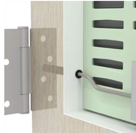
Cable way with intumescent sleeve
