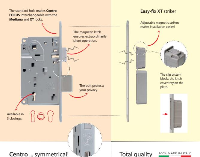
The position of the handle hub and the key, symmetrical in relation to the centre of the panel, make the lock non-handed. The number of panels in stock is considerably reduced.
